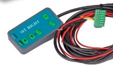
The leveller is self-calibrating and checks the basic settings of the unit every time it is powered and corrects the settings if that is necessary.
